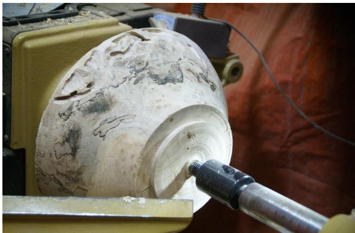
Blank mounted between centers, shaped, and tenon turned.
