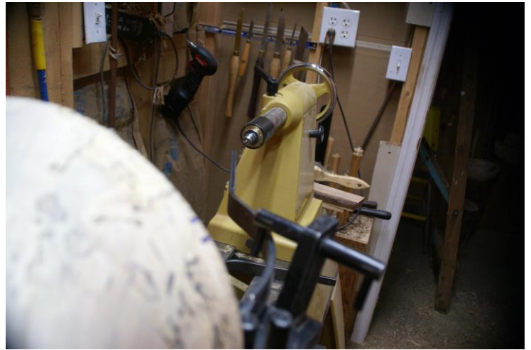
Middle curved cutter aligned for beginning of cut.
