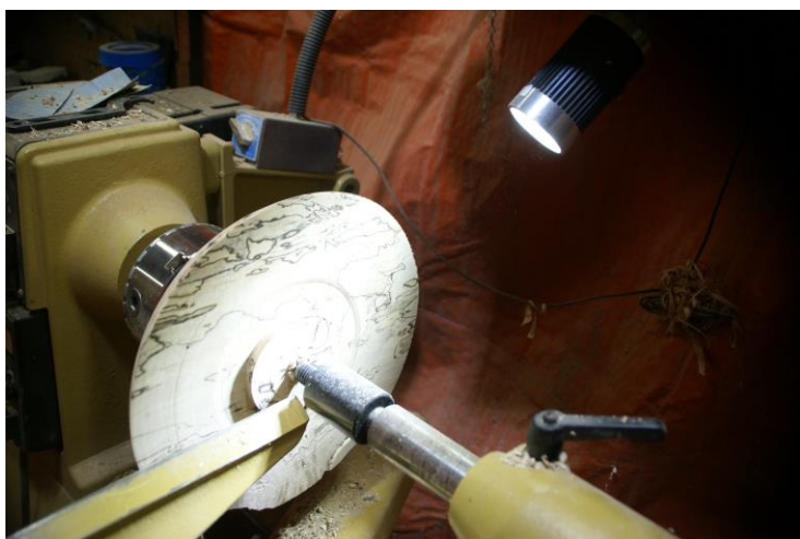
Top turned flat and small tenon made on interior bowl.
