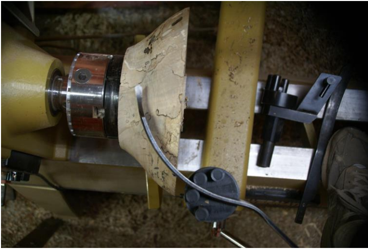
Middle curved cutter tested for fit. (This one was best.)
