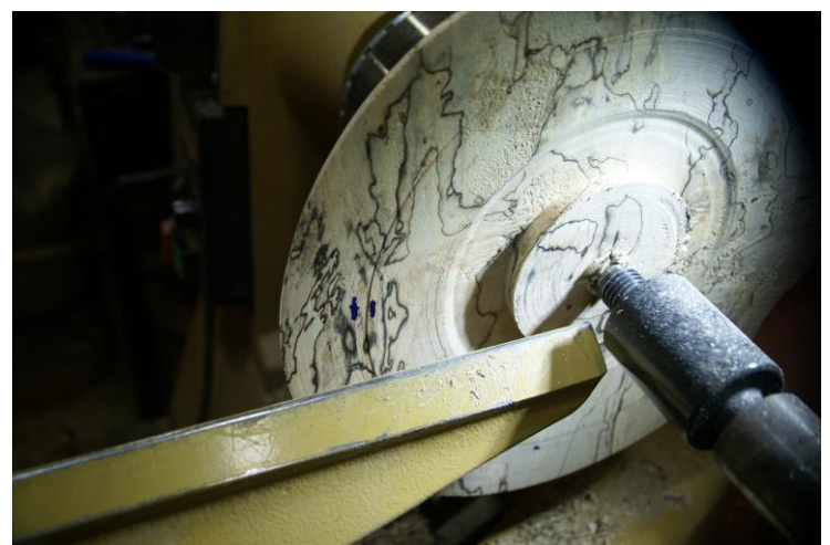
Marks made where cut is to be made.
