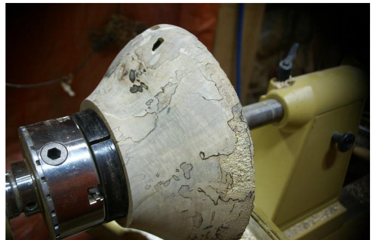
Bowl reversed and mounted in a chuck.
