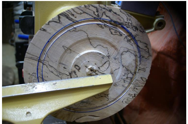
Marks on face extended and groove cut into face where cutter will begin.
