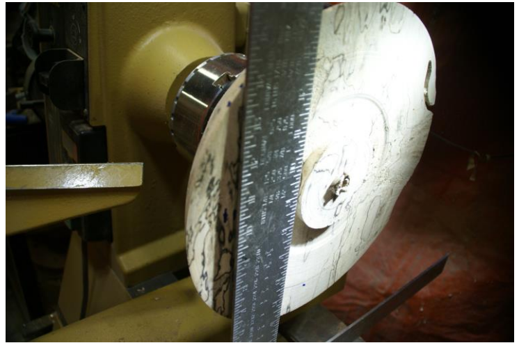
Use square to mark edge of blank above marks on face.
