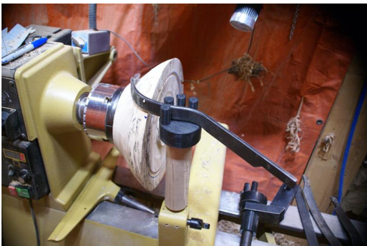
3d Printed head supported by dowel in banjo. Cutter is sitting on top of bowl and 3d printed piece.
